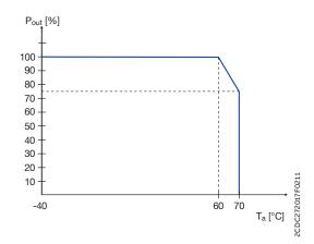
Characteristic curve of temperature at rated load
