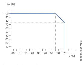
Characteristic curve of temperature at  $U_{\text{out}}$
