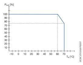
Characteristic curve of temperature at  $\mathbf{U}_{\text{out}}$
