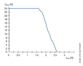
Characteristic curve of output at  $T_a = 25$  °C
