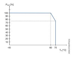
Characteristic curve of temperature at rated load
