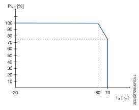
Characteristic curve of temperature at rated load
