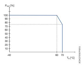
Characteristic curve of temperature at rated load
