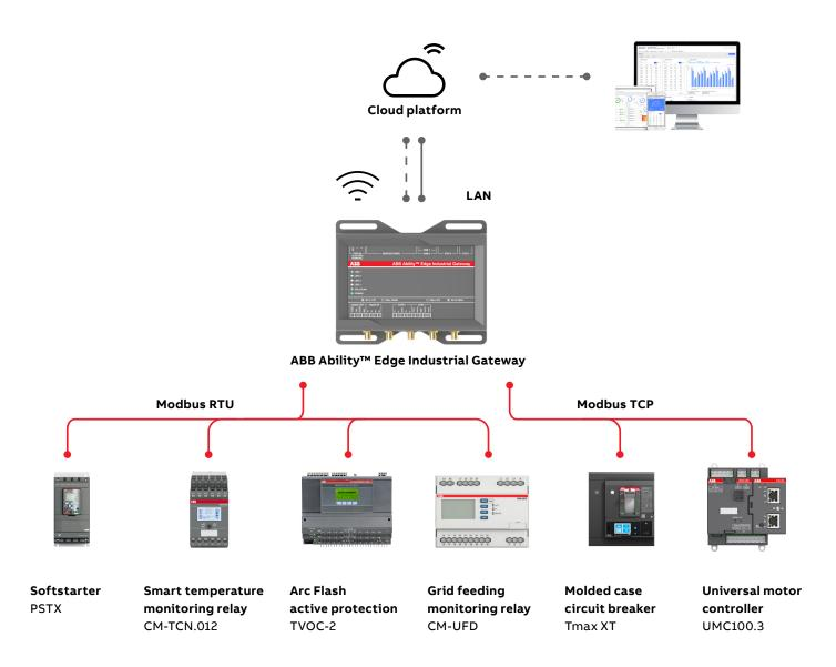
Integrate a range of devices like circuit breakers, motor controllers and the new CM-TCN.012 monitoring relay into the ABB Ability<sup>TM</sup> Energy Manager and ABB Ability<sup>TM</sup> Asset Manager. It is a state-of-
