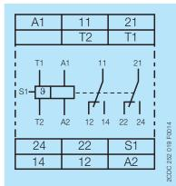
A1 – A2 11 – 12/14 21 – 22/24 S1 – T2 (jumpered) T1 – T2 Control supply voltage 1st c/o (SPDT) contact 2nd c/o (SPDT) contact Automatic reset Measuring circuit
