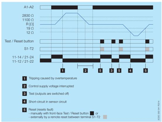
Manual or remote reset (= non-volatile fault storage)
