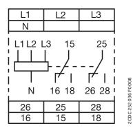
L1, L2, L3, N Control supply voltage = measuring voltage
