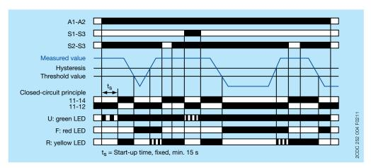
Insulation resistance monitoring with fault storage, manual reset
