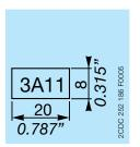
MAR.01 - Marker label for devices without DIP switches
