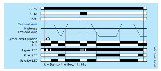
Insulation resistance monitoring w/o fault storage, auto reset
