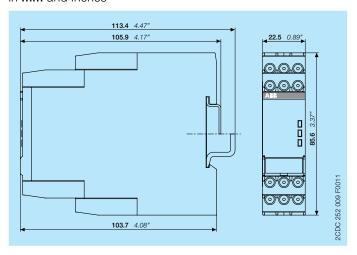
CM-IWS.1 - Insulation monitoring relay
