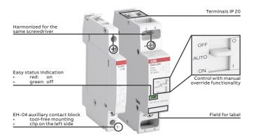
ABB's installation contactor range comes with a host of features to make installation and maintenance easier.
