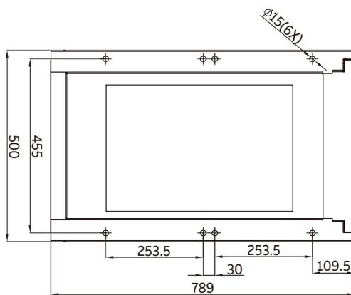
SafePlus与10 kV PTC柜底板安装图
