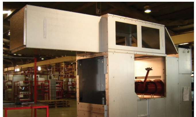
The completed assembly of arc vent duct for middle panel with flap channel (total height of the switchgear is 2662 mm)
