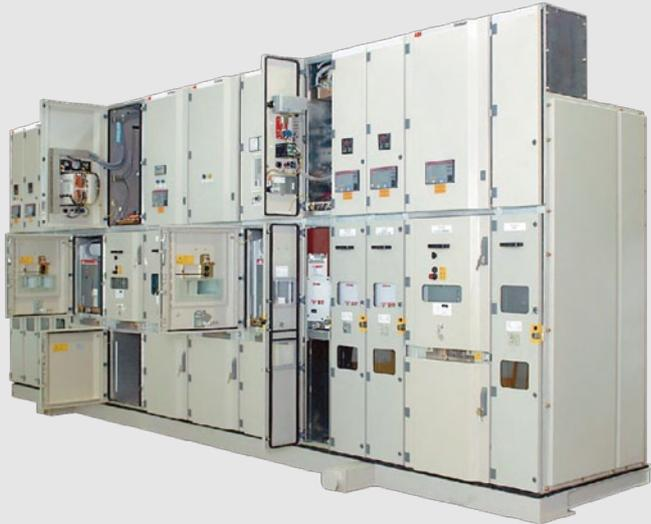
UniGear ZVC is an optimized solution for switching of motors and transformers in networks rated up to 7.2 kV, 4000 A and 50 kA fault level.
