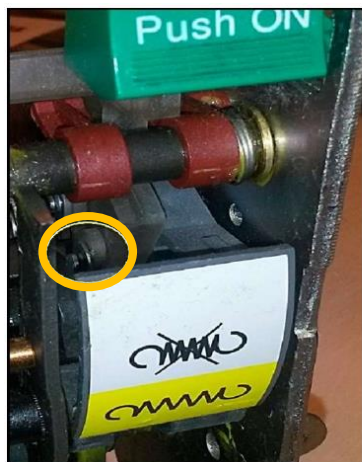
Figure 22 - Antireclosing lever and closing hook
