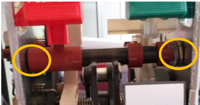
Figure 21 - Closing shaft and opening hook 2
