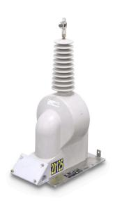
The TJO 7 is a robust voltage transformer that uses ResiVolt™ transient resistant technology for line-to-ground applications, with an enhanced design for operation in renewable and frequent line switching installations. The TJO 7, CBS modification is an alternative to types VOG-15B, VOG-20B and VOG-20BR.
