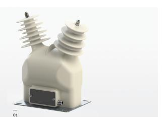
VOL-24L double pole voltage transformer is cast in hydrophobic epoxy resin (HCEP), capable of withstanding outdoor environmental conditions and designed for insulation voltages up to 24 kV.
