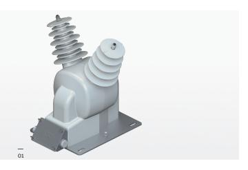
VOL-24 double pole voltage transformers are cast in cycloaliphatic epoxy resin (HCEP), capable of withstanding challenging outdoor environmental conditions and are designed for voltage classes up to 24 kV
