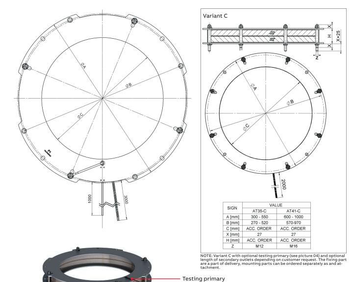
NOTE: The Length of an outlets (testing primary, secondary outlets) is optional and depends on customer request. The fixing parts are a part of a delivery, mounting parts can be ordered separately as an attachment.
