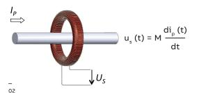
In all cases, a signal that represents the actual primary current waveform is easily obtained by integrating the transmitted output signal.
