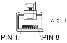
PIN 1 - COIL START (S1) PIN 2 - COIL END (S2)
