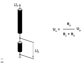
In all cases, the transmitted output signal reproduces the actual waveform of the primary voltage signal.
