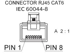
PIN 4 - COIL START (S1) PIN 5 - COIL END (S2)
