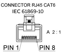
PIN 1 - COIL START (S1) PIN 2 - COIL END (S2)
