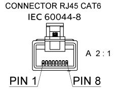
PIN 4 - COIL START (S1) PIN 5 - COIL END (S2)
