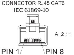
PIN 1 - COIL START (S1) PIN 2 - COIL END (S2)
