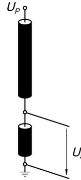
$$U_s = \frac{R_2}{R_1 + R_2} U_p$$
