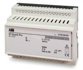
VT Guard Pro is an security device that protects medium voltage inductive voltage transformers against ferroresonant oscillation. Ferroresonance can arise in ungrounded power networks or in the networks where is not directly grounded neutral point. It is designed to be used in opendelta connection of three single-phase voltage transformers. VT Guard Pro (Pro-D) fully replace dumping resistor and save space in customer application.
