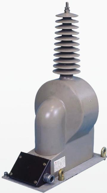
The TJO 7 single-pole insulated voltage transformers are cast in outdoor epoxy resin and are designed mainly for insulation voltages up to 40.5 kV. Insulation voltages different from the above are to be the subject of an agreement between the manufacturer and the customer. Alternative insulation voltages are available to special order. Standard transformers incorporate an overvoltage factor of 1.9  $U_n/8$  hrs.
