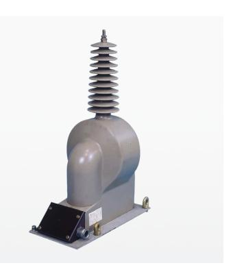
The TJO 7 single-pole insulated voltage transformers are cast in outdoor epoxy resin and are designed mainly for insulation voltages up to 40.5 kV. Insulation voltages different from the above are to be the subject of an agreement between the manufacturer and the customer. Alternative insulation voltages are available to special order. Standard transformers incorporate an overvoltage factor of 1.9 Un/8 hrs.
