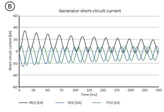
Failure location A: System-fed fault Fast decaying DC component Failure location B: Generator-fed fault Slowly decaying and raised DC component results in delayed current zero
