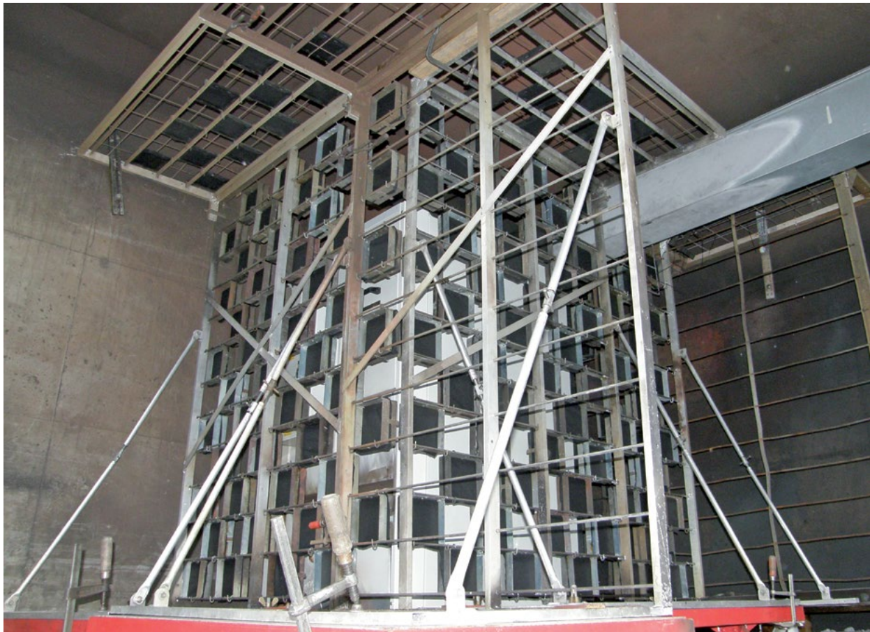
Setup for an internal arc withstand test
