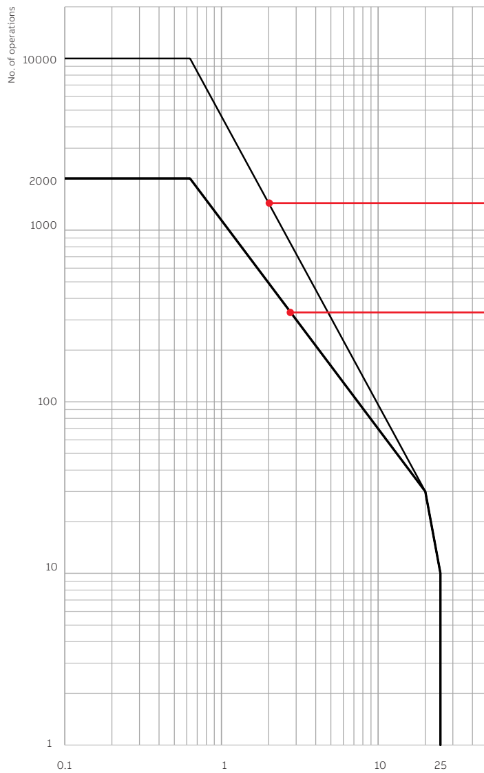
SafePlus V25 High duty - 12kV (VG4 - M1/M2)
