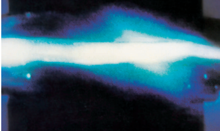
Fig. 2.8: vacuum arc between contacts
