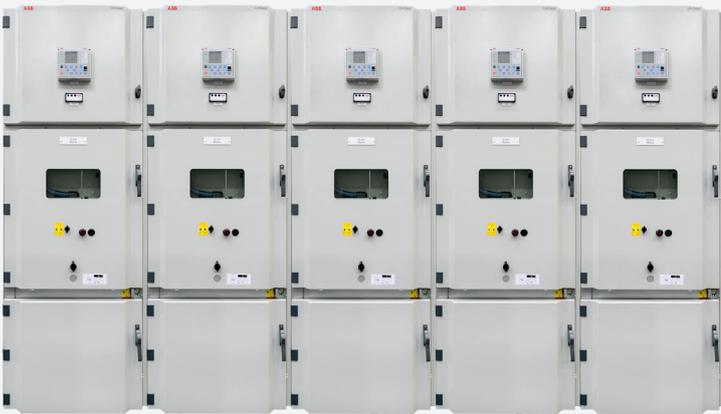
Each panel consists of two single units connected in double busbar arrangement. They can be equipped with circuit-breaker or contactor as well as with all the accessories available for the conventional units of the switchgear. Each panel is provided with a cubicle to take the auxiliary instrumentation, placed in the upper part.
