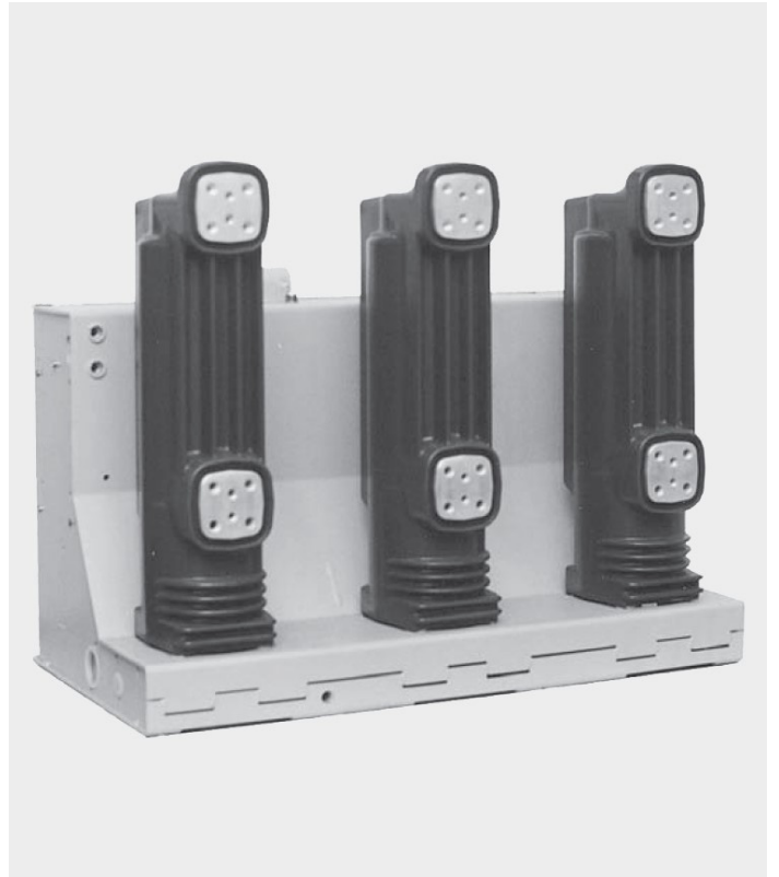
Figure 9/2: Vacuum circuit breaker, type VM1, high-current, for fixed installation, 12 kV, 1600...2000 A, 40 kA, pole side
