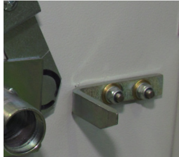
Lock installed on the inner side of the door
