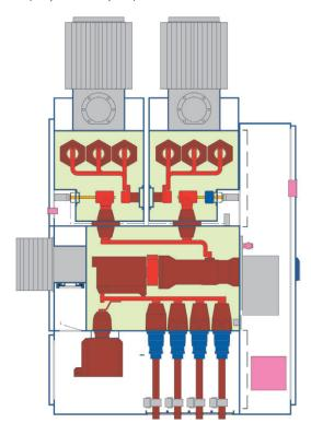
Example of a panel (rated normal current 2000 A) with tall heat sinks on the busbar compartments for a rated frequency of 60 Hz
