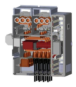
The permissible rated busbar current of the proven switchgear type ZX2 is increased by parallel connection of the two busbar systems. The two physical busbar systems are combined electrically into a single busbar system. The current carrying capacity of the busbar in this application is up to 5000 A under standard conditions.
