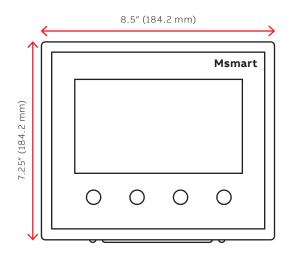
8.5" × 7.25" × 1.75" (H × W × D) 215.9 × 184.3 × 44.5 mm (H × W × D) ABOUT MSMART
