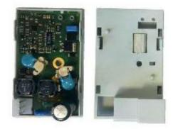
During manufacture of the electronic board, the main operating program for the SmartCS is flashed on to the processor and can never be updated or changed for the life of the coil except for 12 configurable parameters. This ABB proprietary firmware performs all on board monitoring and control functions during operation. The functions performed for increased reliability are as follows:
