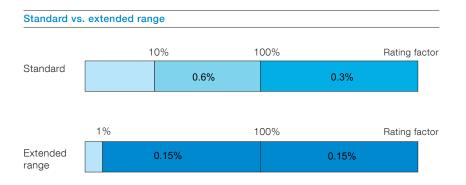
ABB's extended range design delivers high accuracy and stable performance over a wide load swing, making it a great fit for variable load applications. Accuracy is guaranteed to be +/- 0.15% from 1% of nominal current through rating factor. ABB's extended range units deliver savings through improved accuracy metering and reduced inventory.
