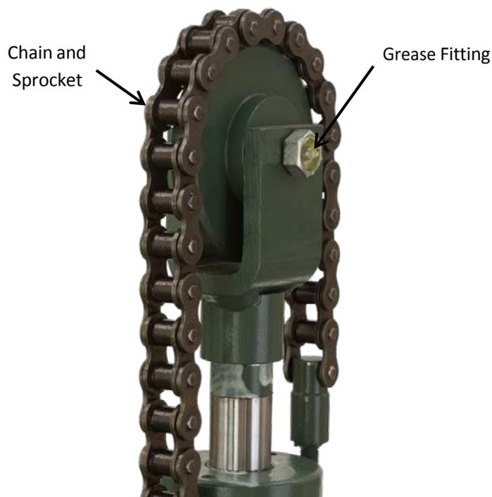
*Figure 32: Lift Truck chain and sprocket*
