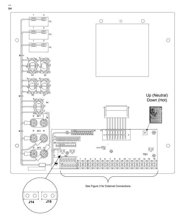
Figure 05.TCC300M2270B wiring harness with optional SCAMP™ auto/manual pushbutton switch, voltage reduction and scada cutout switches
