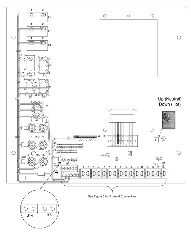
Figure 06. Tapchanger control and LTC backup control interconnections
