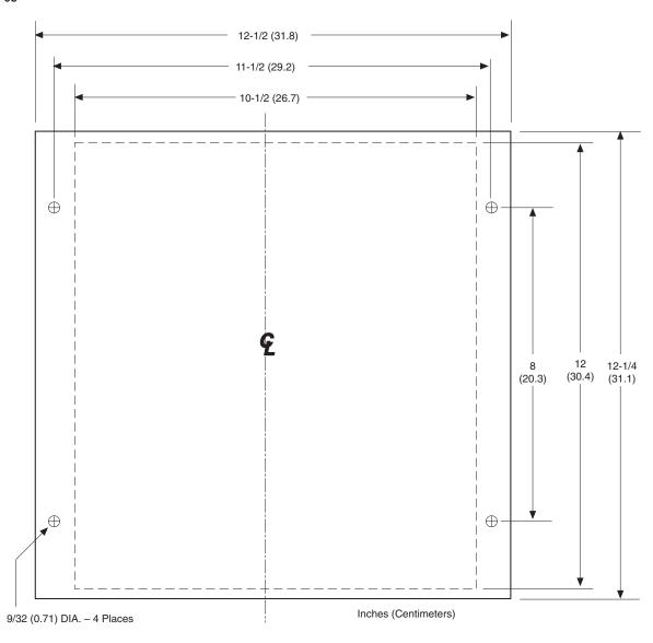
Figure 09. 19" rack mount adapter panel dimensions
