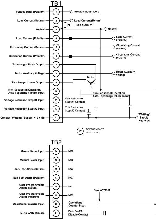
▲ Warning Open CT secondary will result in high voltage at CT terminals. Death, severe injury or damage to equipment can occur. Do not operate with CT secondary open. Short circuit or apply burden at CT secondary during operation.
