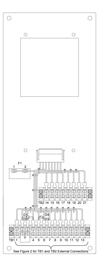
Figure 04. Tapchanger control and LTC backup control interconnections
