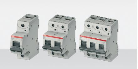
This paper does not cover non-current limiting MCBs ("zeropoint crossing" MCBs). Modern, current-limiting MCBs are typically used for protecting cables/conductors and loads up to 100 A using a combination of thermal and magnetic trip units. The thermal trip unit is based on a bi-metal strip while the magnetic one is based on a solenoid.
