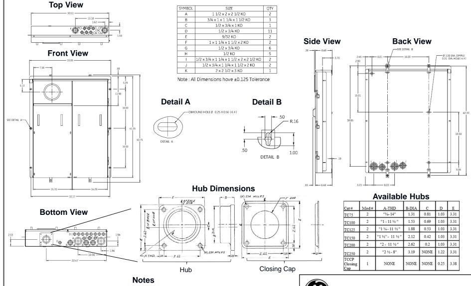
1/2" Studs Provisions for UL Listed One or Two Hole NEMA Mounting Terminals
