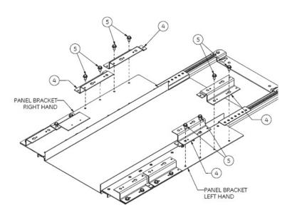
Figure 5. Installation of FB bracket
