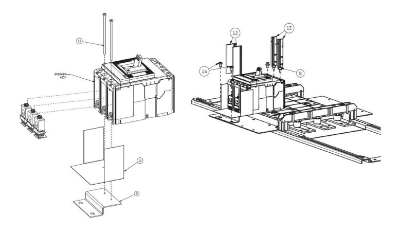
Figure 2. Installation of XT2 three-phase, three-pole breaker subassembly.
