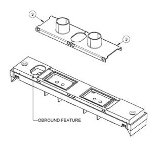
Figure 4. Installation of FB cover
