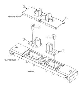
Figure 1. Installation of XT2 spools and covers
