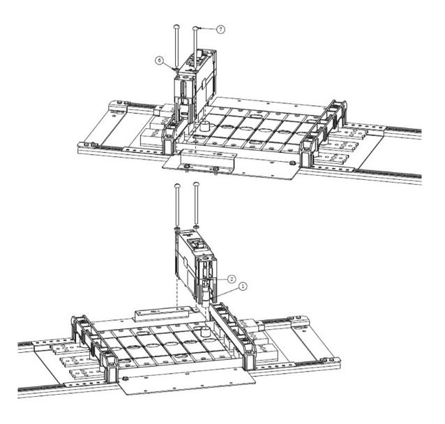
Figure 6. Installation of FB breaker
