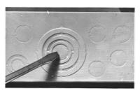
First knock the center knockout inward. The outer rings should be alternately pried up or driven in one at a time.
