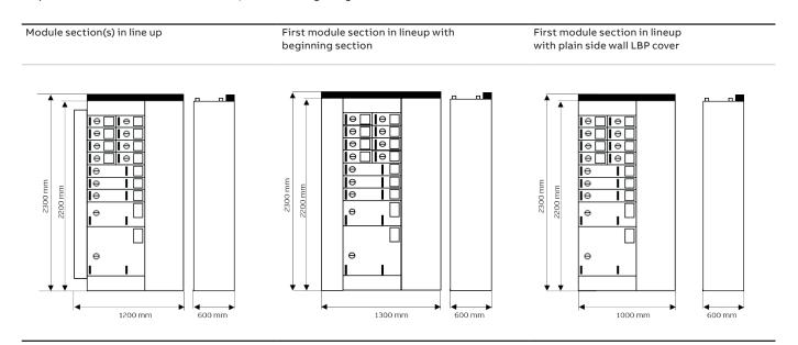
The following representative dimensions are applicable to the NeoGear sections. **DC2BP Section:** Depth: 600 mm\*\*, Width: 500 mm-1050 mm, Height: 2300 mm \*\* excl pagoda cover
