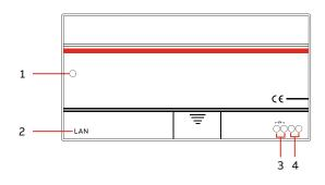
The IP Gateway enables integration of smartphones and devices (iOS and Google's Android™) to the door entry system. The IP-Gateway has a user interface that can be reached via an Internet browser.
