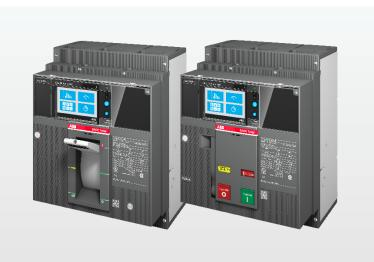
Tmax XT7 — 1200 A frame available up to 600 V UL. MCS, MCP, basic and advanced electronic trip units. Max. interrupt rating of 100 kA at 480 V, 65 kA at 600 V. A powerful package capable of monitoring and controlling distribution.
