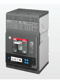
250 A frame available up to 600 V UL. Thermal-magnetic, MCS, MCP basic and advanced trip units. Max interrupt rating of 200 kA at 480 V, 100 kA at 600 V. Advanced electronic trip offer embedded Bluetooth® communication, allowing interaction without direct contact.
