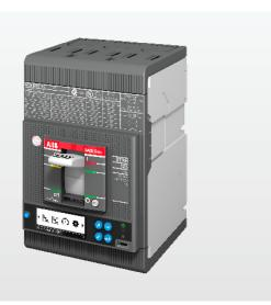
125 A frame available up to 600 V UL. Thermal-magnetic, MCS, MCP basic and advanced trip units. Max interrupt rating of 200 kA at 480 V, 42 kA at 600 V. Electronic trip units, high interrupt ratings, communications and embedded logic.
