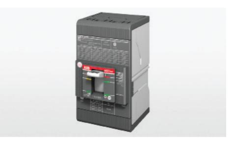
125 A frame available up to 480 V Delta UL. Thermal-magnetic, MCS and MCP trip units. Max. interrupt rating of 65 kA at 480 V. Offers savings versus 600V rated systems in most distribution applications.
